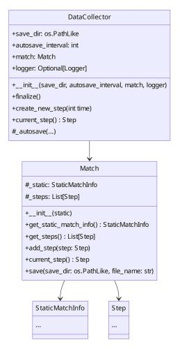
Figure 4.1.: UML class diagram of the high-level classes DataCollector and Match. StaticMatchInfo and Step have been simplified, as the details will be shown later.
