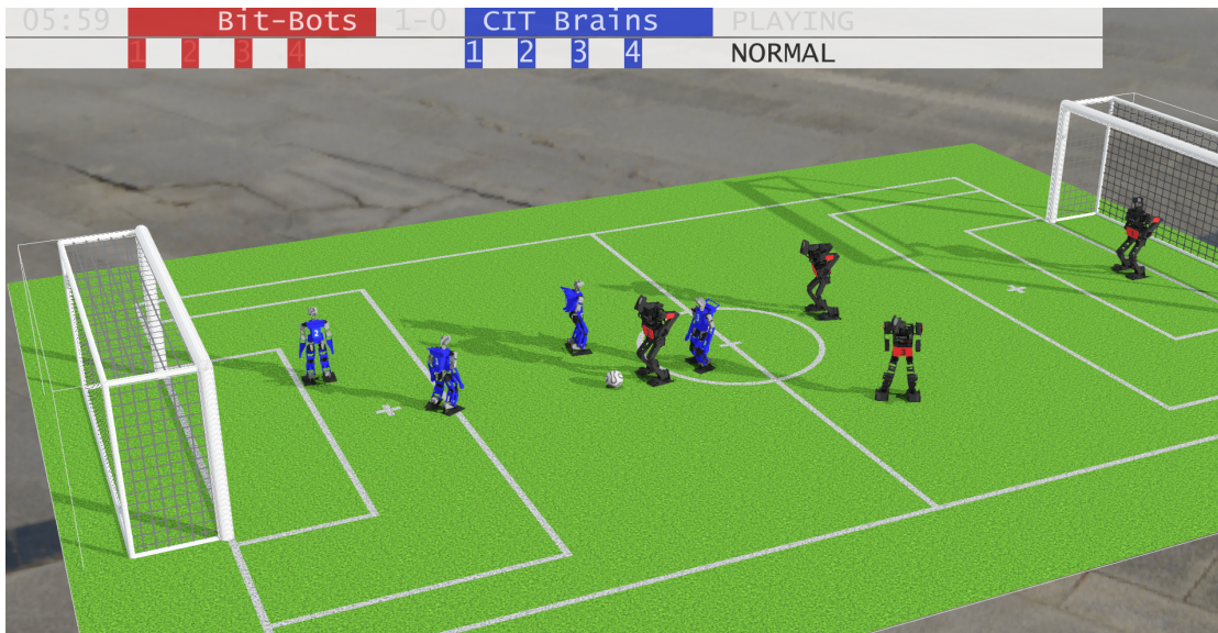
Figure 1.1.: Typical scene from the Humanoid League Virtual Season. Four robots per team compete in the simulated soccer competition based on the rules of the RoboCup Humanoid League. Only simulated sensor information and team communication can be used to perceive the environment. The robot platform playing in red is used in this thesis.
