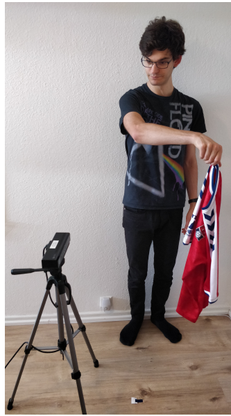
Figure 4.2.: Exemplary image of the data collection process and setup. The user holds the piece grasped at a single position in front of the Kinect camera. A distance of 0.6m to 1m between the camera and the piece is maintained with the help of markers on the floor.
