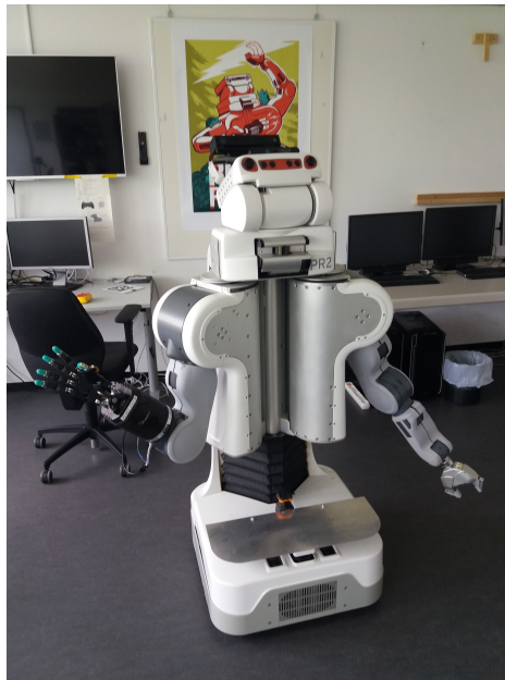
Figure 4.1.: The Willow Garage PR2 with the Shadow Dexterous Hand attached to the right arm and the standard PR2 gripper on the left arm.
