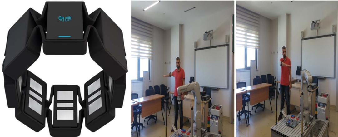
Figure 2.3: **Left:** The Myo armband leveraged to operate a 6-DOF manipulator. It is used to measure electromyographic signals from the user. Then, the data gets transmitted wirelessly over Bluetooth. **Middle/right:** The operator, wearing the Myo armband on his right arm, controls the robot wirelessly by only moving his arm. [25]
