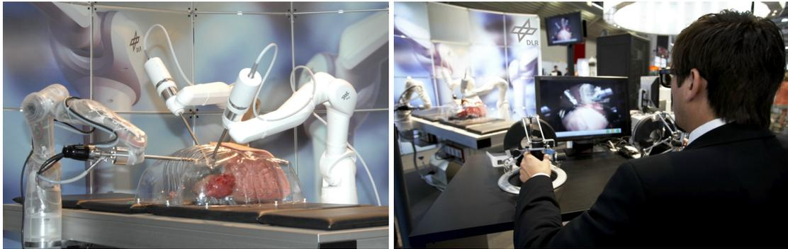
Figure 2.5: **Left:** Three robotic arms with each 7 degrees of freedom help in minimally invasive surgeries. They are equipped with two surgical instruments and one stereo endoscope. Force torque sensors on the surgical instruments help to give feedback to the surgeon. **Right:** The operator controls the robotic system with two input devices. The stereo display provides visual feedback coming from the endoscope. [31]
