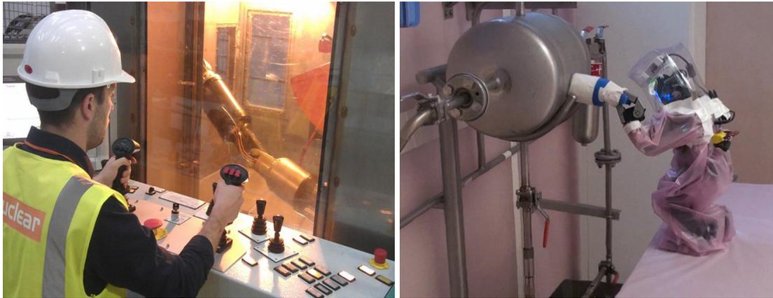
Figure 1.2: Nuclear decommission involves working with highly radioactive material. Letting humans carry out this work directly should be avoided as much as possible. **Left:** A teleoperated 6 DOF robotic arm with a payload of 100kg controlled by two joysticks [4]. It can be used to move contaminated material while the operator stays at a safe distance. **Right:** A DARwIn-OP was sent to take smears and assess object contamination [5].
