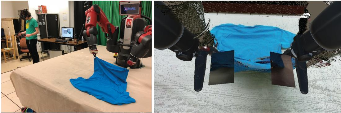
Figure 2.2: **Left:** The user controls a Baxter using virtual reality and ROS Reality. The task is to fold a shirt. **Right:** The users view through the VR headset. It shows a combination of a point cloud from the scene and a mesh model of the robot. [22]
