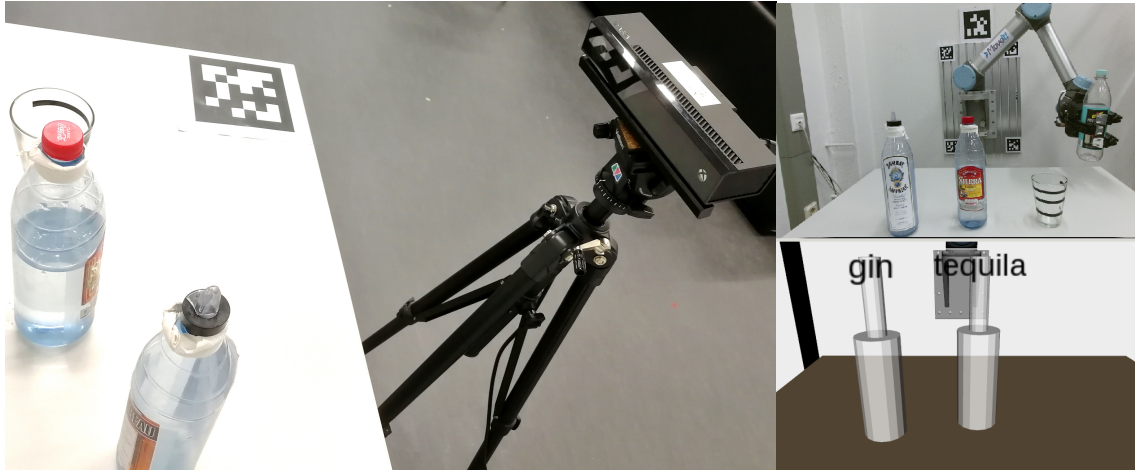
Figure 1.2: Camera recognizing and locating bottles
