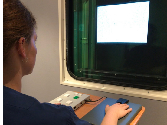
Fig. 1. The original human visuo-tactile discrimination experiment. The participant looks for a (four-dot) visual pattern on the monitor and feels a haptic pattern generated by a Braille actuator on the index finger of the right hand. The participant then decides whether both patterns are the same or different, and presses the green or red button accordingly. The task is made more difficult by blending the visual pattern in the background noise and by reducing the actuated pin height of the tactile display.
