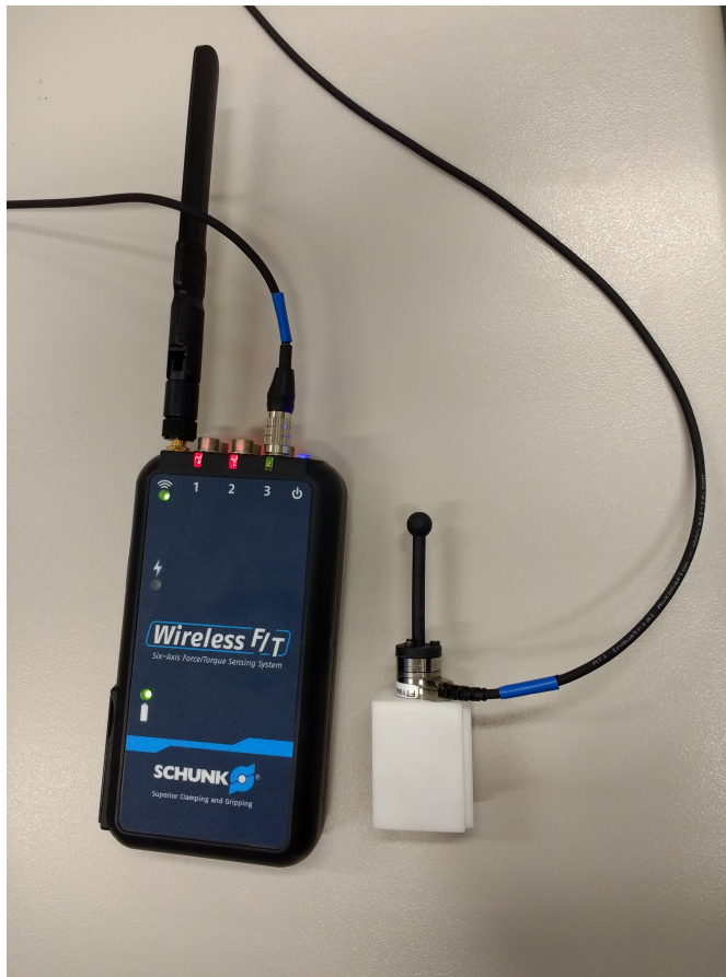
Figure 3.5: The pictured ATI/Schunk Wireless Force/Torque Unit is connected to the ATI nano17e transducer. The green LEDs show active status of the transducer slot 3, the device running in battery mode and active wireless LAN.
