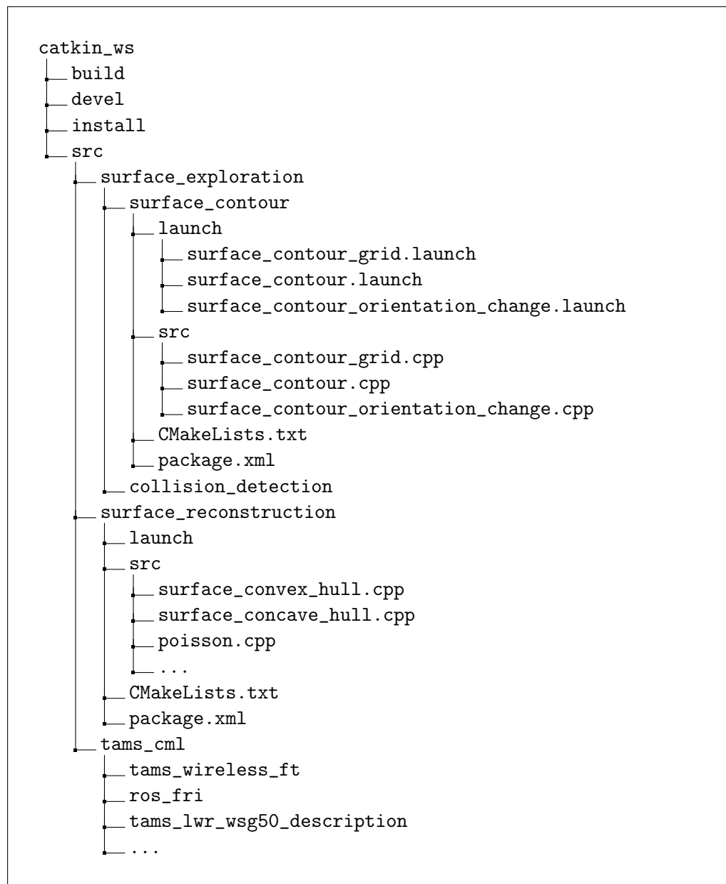
Figure 5.2: The catkin workspace used for the surface exploration and reconstruction is shown. Thereby a separation between the packages has been realized to modularize functionality to generate better maintainability and ease reusability.
