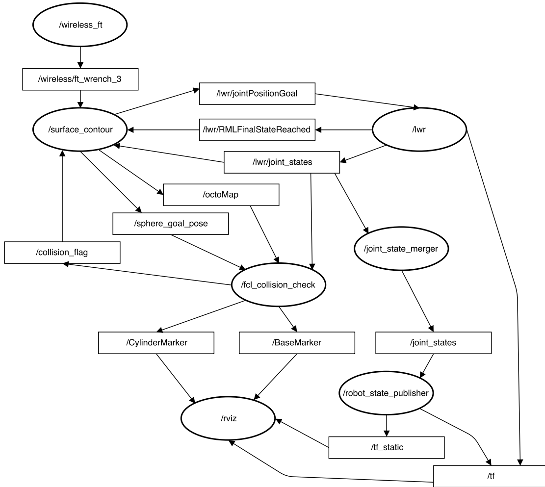
Figure 5.5: The ROS computation graph shows the used nodes and topics for surface exploration and the 3D visualization in rviz. The topics are illustrated in rectangles whereas the nodes are illustrated in ellipses. The arrows between the elements show the communication via topics based on publisher/subscriber architecture.
