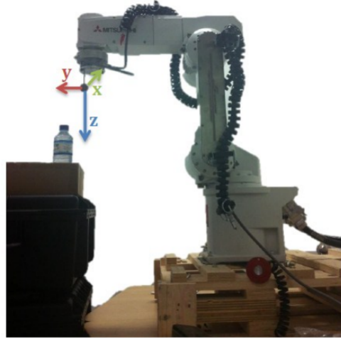
Figure 1.3: The experimental setup of Hussein et al to blindly perceive the shape of a bottle with force/torque sensor and a 6-DOF manipulator.
