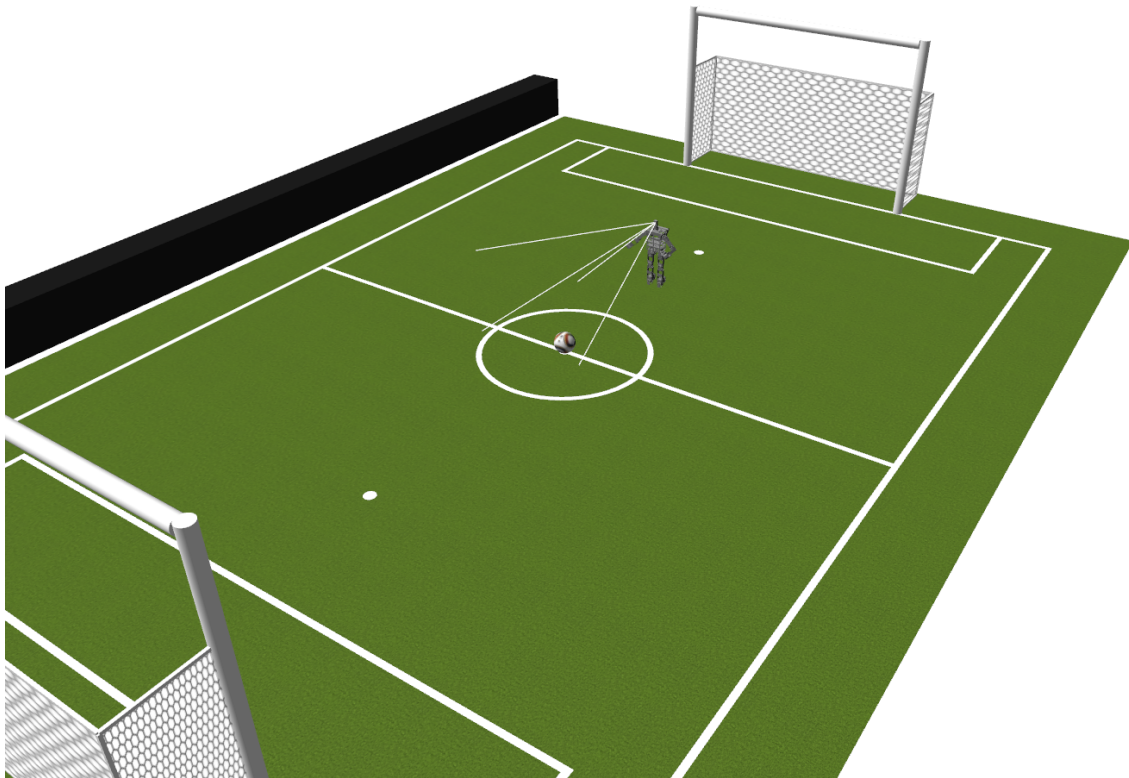
Figure 5.2: The Humanoid League environment which was extracted from the Nimbro code base. The Minibot robot was integrated using the modeled URDF, cp section 5.2.3. The lines in front of its head visualize the robot’s field of view.
