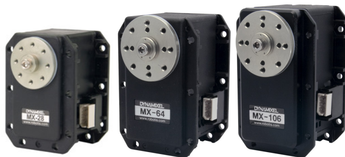
Figure 3.2: The MX-28T, MX-64T and MX-106T servos [6]. All three are controlled by the same TTL bus protocol. The only difference is the maximal torque.
