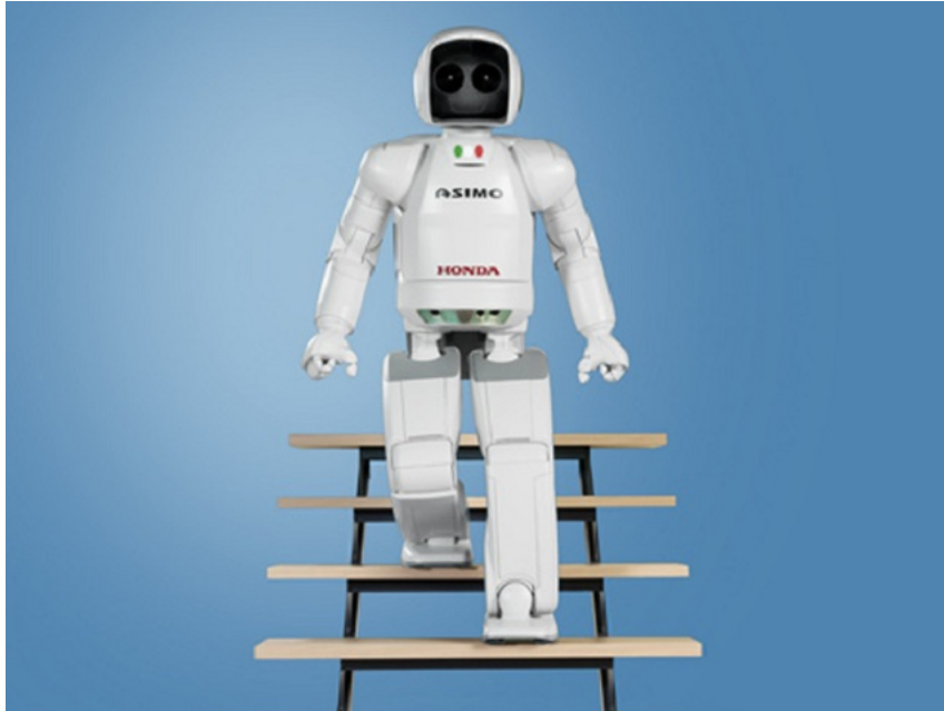
Figure 2.3: The Asimo robot walking on a flight of stairs [2]. The algorithm was adapted to this specific stair size, therefore it is not applicable in the real world. This transfer from the lab environment to the real world is tried to be achieved in RoboCup by enforcing realistic testing conditions in which teams have to prove their performance.
