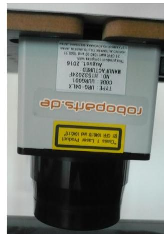
(c) This is the laser low-frequency sensor, that is mounted on the TurtleBot.
