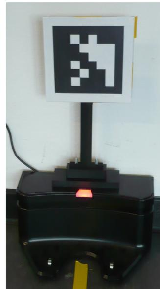
(c) Shows the retainer on top of the docking station.
