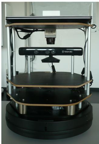
(a) The Kobuki TurtleBot with the Kinect and the mounted laser sensor
