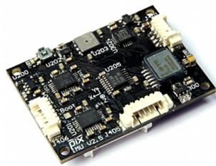
(b) This figure shows a typical IMU. It is a PIXHAWK IMU that is described in [3].
