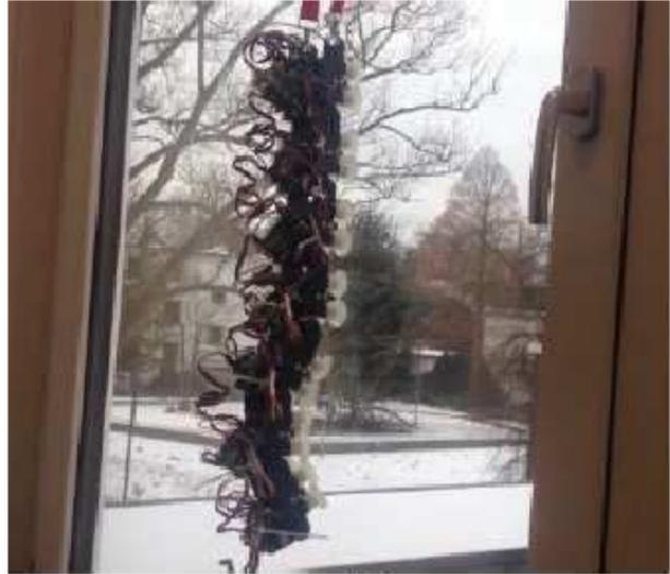
**Figure 3.7:** Climbing caterpillar-like robot (Chen et al. [11])
