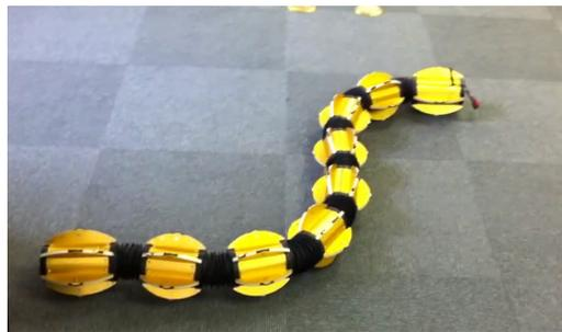
**Figure 3.2:** ACM-R5H is an amphibious snake robot. Efficient locomotion on land by using wheels is provided as well as swimming and diving in water. In both cases locomotion is generated by wavelike motions of the body. (HiBot [26])
