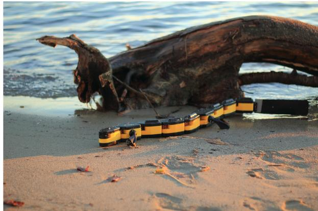
**Figure 3.5:** AmphiBot is based on hyper-redundant chain of identical modules but has some special parts to increase its capabilities. There are four legs and a tail. Inspired by salamanders this amphibious robot is designed to swim and crawl in a robust way. (École polytechnique fédérale de Lausanne [57])
