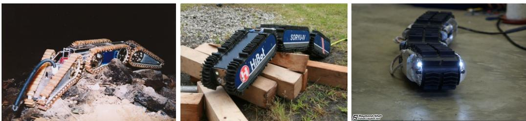
**Figure 3.3:** Series of Soryu robots consist of three modules driven by tracks. They are designed for tasks in rough terrain. Single modules can be autonomously disconnected or connected. These special joints are powerful enough to rotate or lift connected modules. (HiBot [26])
