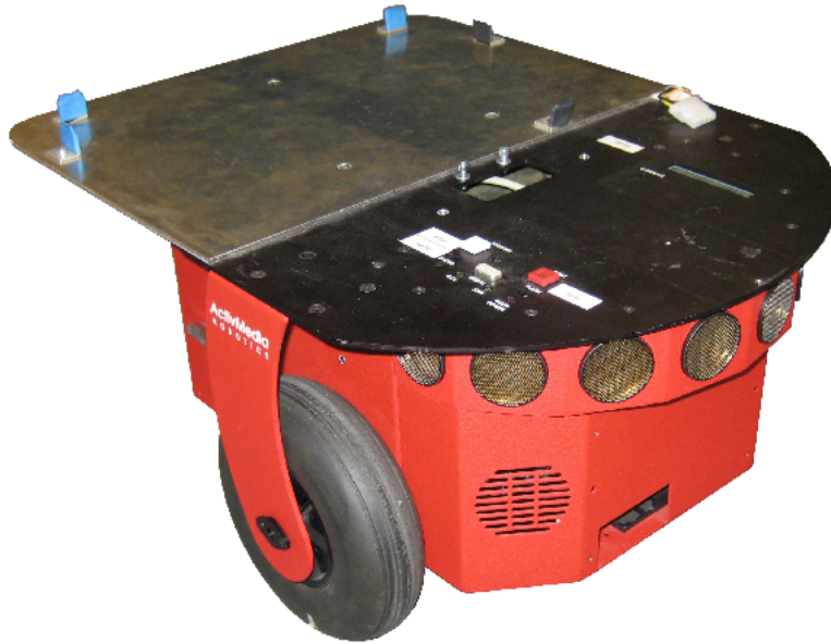
Figure 3.1: The Pioneer 2 DX robot. The original robot is slightly modified by extending the platform on its top. The picture also shows the sonar sensors mounted on the robot's front. (Image from [8])
