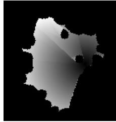
Figure 5.8: Cost map. The brighter a point on the map is the higher are the costs of moving there. It is easily visible that some points are only reachable by an indirect traveling route over certain landmarks. The current robot position is also easily detectable in this image.
