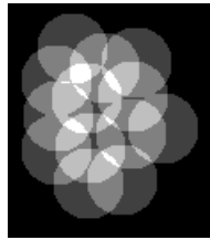
Figure 5.9: Knowledge map. The brighter a point on the map is the higher is the knowledge already obtained for this point. The scan positions of the robot are easily detectable in this image.
