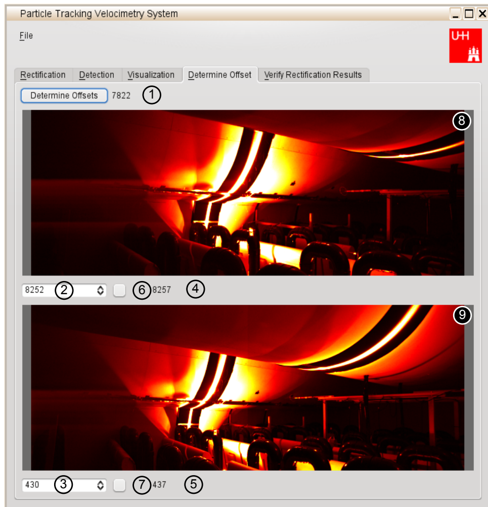
Figure 8.5: Screenshot of the widget, which assists the user in determining the frame offset between both cameras.
