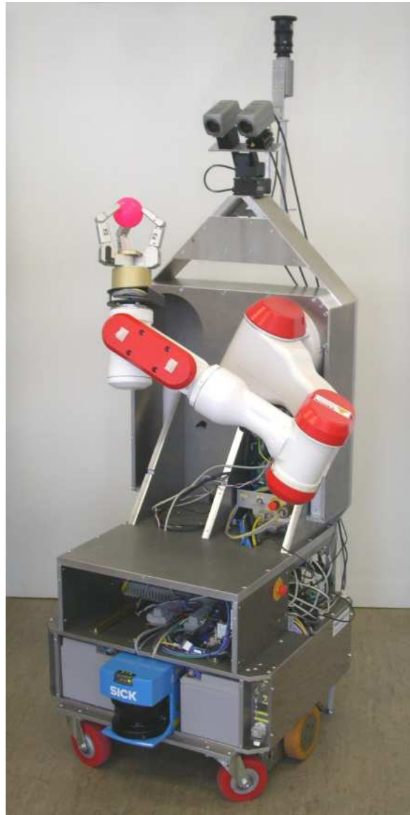
Figure 1.1.: The robot TASER The laser range finder is the blue box at the bottom with “SICK” on it The cameras can be seen at the top
