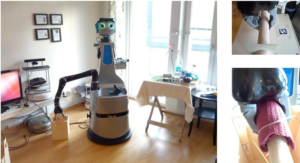
Figure 34: The photo shows grasping the prototype basket that will be used for the garbage scenario (left). AprilTag markers are put onto the object to improve object identification and pose estimation. In this case, the new side camera is used for detection, and the head is idle and can point straight ahead. Closeup of a soft cylindrical handle that is a good fit for power-grasps with the Jaco hand (right).
