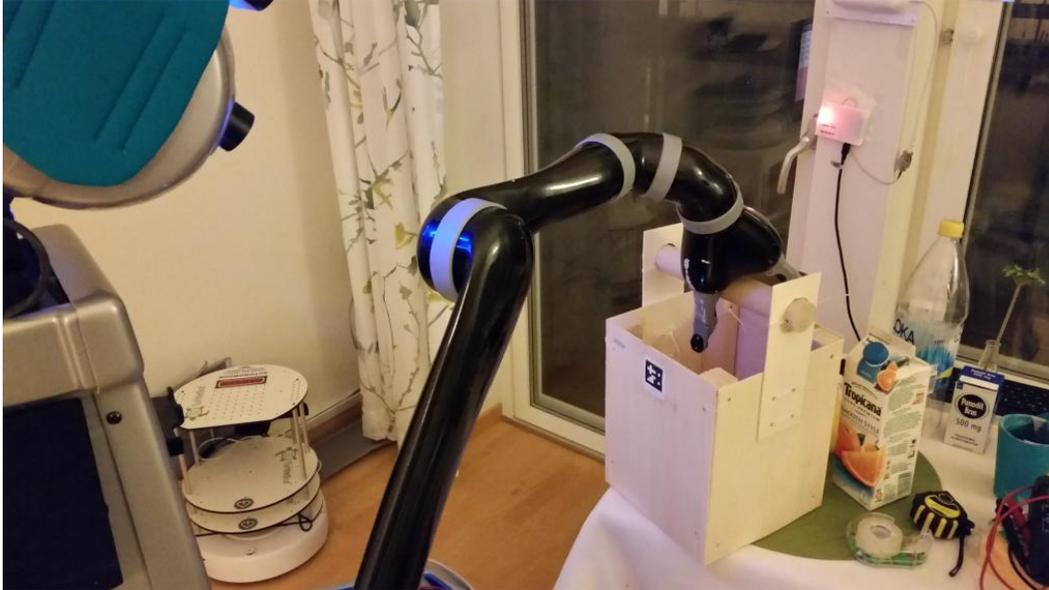
Figure 26: Object manipulation test in Angen, Örebro. Doro is grasping the prototype box for the garbage and laundry scenarios. As the wood lacks any visual texture suitable for SIFT feature matching, an AprilTag fiducial marker has been placed on box. Despite the small size of the marker tag, marker detection and identification are very reliable, and pose estimation errors are usually well below 1 mm position error.
