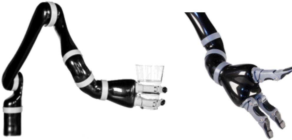
Figure 9: The 6-DOF Jaco arm with integrated 3-finger gripper, and a close-up of the three-finger gripper.
