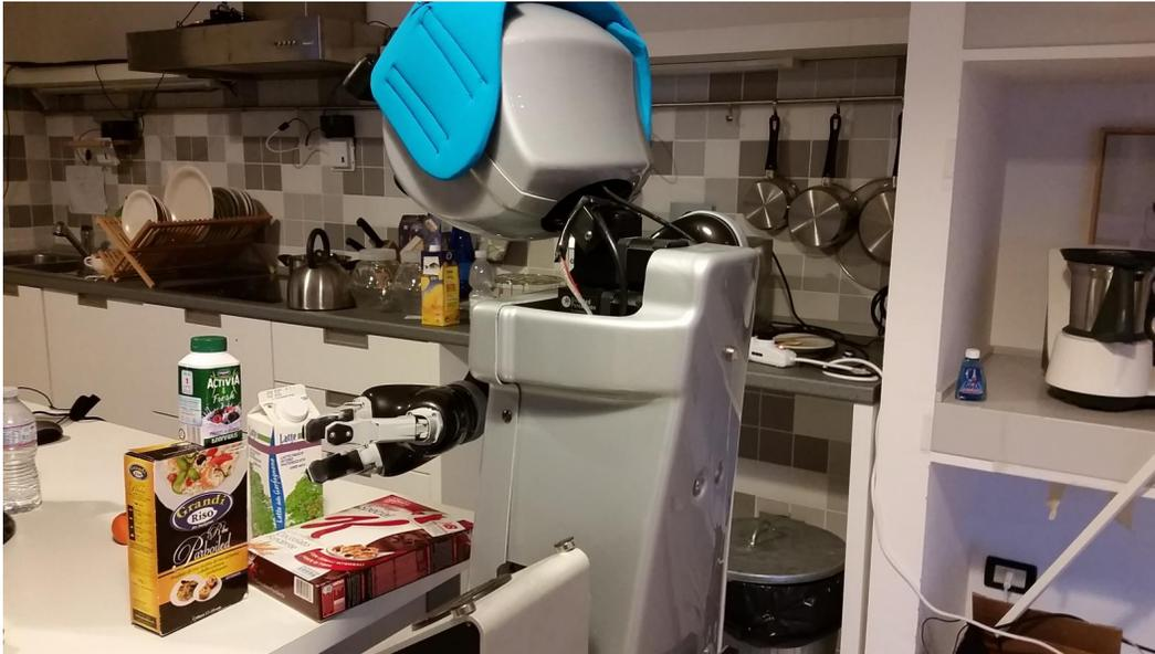
Figure 24: Object manipulation test in the DomoCasa living lab, Peccioli. Doro is looking at a cluttered table scene with objects that have been trained with the SIFT object recognition back-end. Note that the Jaco arm is still in the safe home position used for driving around and as a start position for manipulation. The arm is just outside the camera image.
