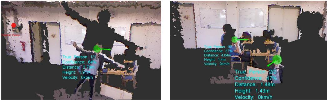
Figure 27: Typical output of the ROS person\_detector module. The algorithm first performs a ground-plane detection to identify the floor and then searches for people-sized clusters in the point-cloud generated from the Kinect/Xtion camera. A pre-trained SVM is used to classify the clusters, and the estimated head position  $(x,y,z)$  and motion are published to ROS. The algorithm detects standing as well as sitting people. [12].
