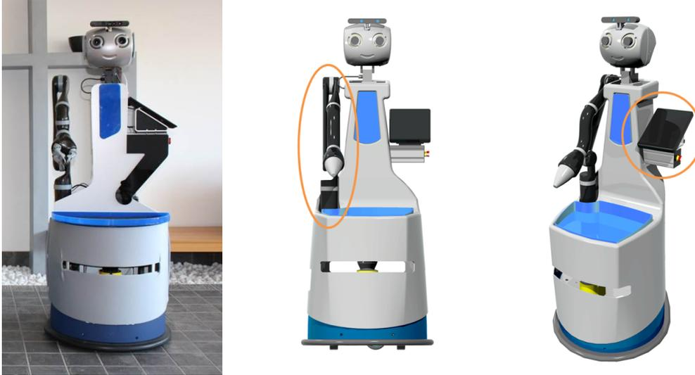
Figure 4: Photos of Domestic Robot for the first experimental loop (left) and sketch of the updated design for the second experimental loop with the new arm position and changed iPad tablet orientation highlighted (right).
