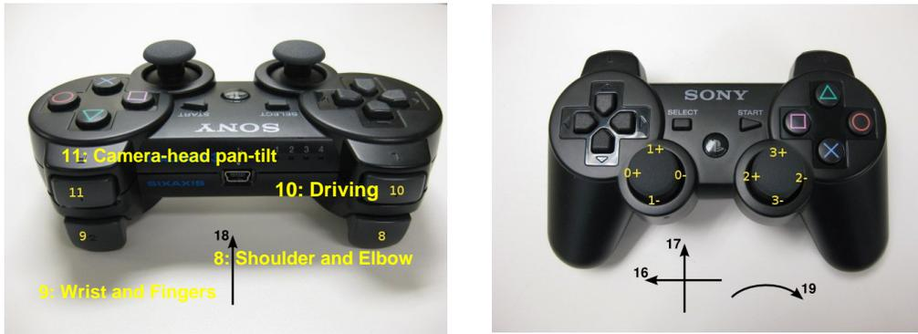
Figure 19: The Sony Sixaxis joystick used in the *doro\_sixaxis\_teleop* node. The labels indicate the axes and button numbers used by the *ps3joy* joystick driver for ROS.
