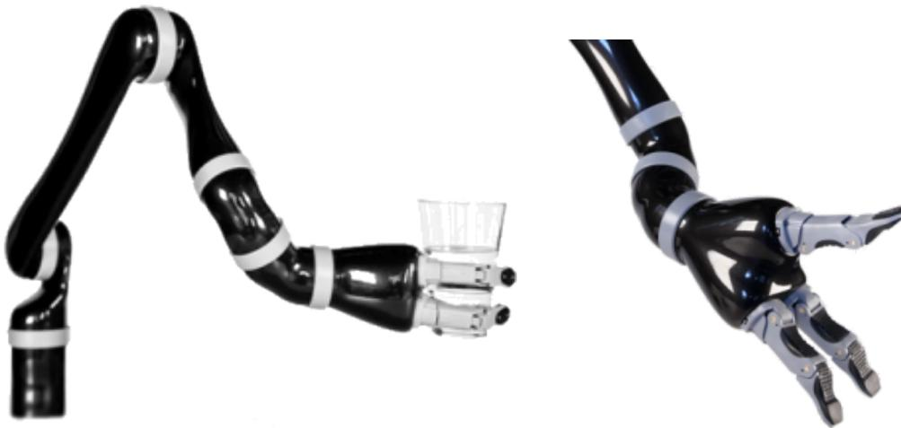
Figure 6: The 6-DOF Jaco arm with integrated 3-finger gripper, and a close-up of the three-finger gripper.
