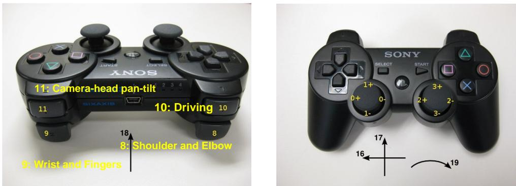
Figure 14: The Sony Sixaxis joystick used in the *doro\_sixaxis\_teleop* node. The labels indicate the axes and button numbers used by the *ps3joy* joystick driver for ROS.
