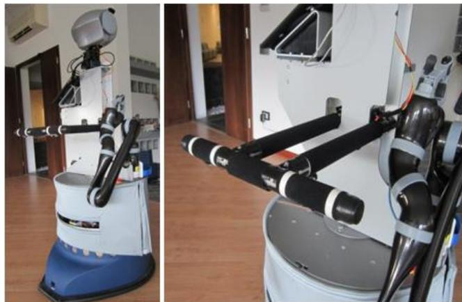
Figure 5: The domestic robot is equipped with an horizontal handle, located on the back of the robot at a fixed height. Two buttons are located on the left and right side of the handle so pushing them the user can drive the robot forward, left and right. In this way the domestic robot provides indoor walking-support to users with limited mobility.
