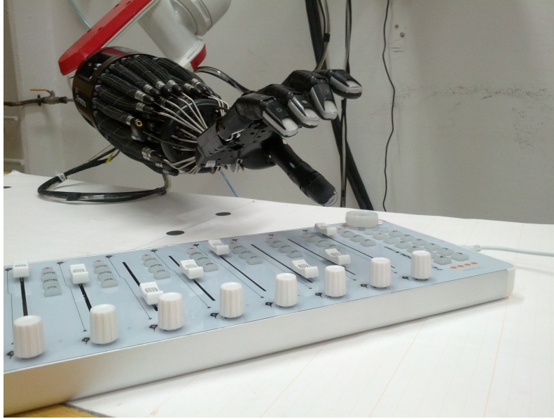
Figure 3: The iControlsPro MIDI controller is a low-cost input device for audio workstation software. It provides motorized faders plus a set of buttons and knobs, and has been used by us in two functions: First, as an efficient human-interface device for interactive hand control, and second, for tracking the effects of robot motions for exploration learning.
