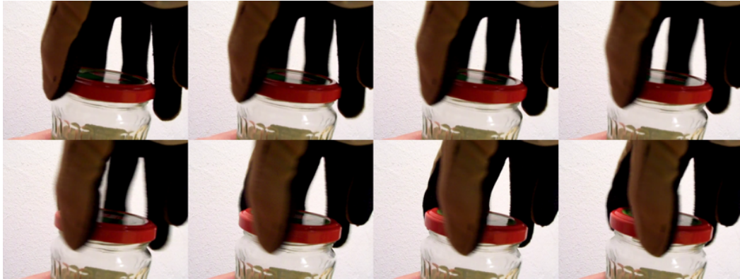
Figure 32: Cylinder rotation learning from screw-cap rotation. A demonstrator wearing a data-glove rotates the screw-cap of a bottle. The thumb, first, middle and ring finger are involved in this application.
