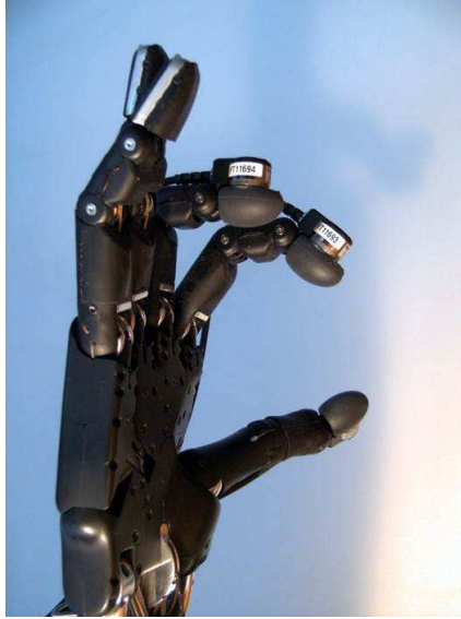
Figure 10: The Shadow Robot Hand equipped with fingertip force/torque sensors ATI NANO 17.
