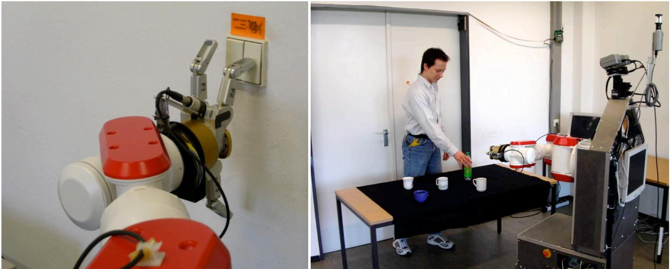
Figure 7: Left: TASER is operating a double-switch. Right: TASER is instructed to grasp a cup by speech and gesture.
