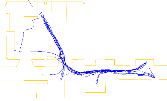
Fig. 4. The 31 trajectories observed during a two-hours experiment. The tracking starts when persons become visible to the sensors and ends when they leave the range of the sensors.
