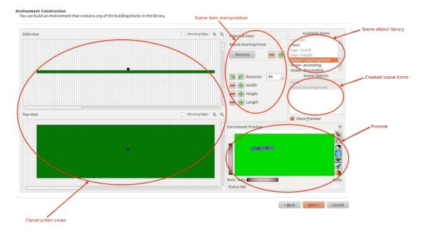
Figure 4.11: The environment editor can be used to create an environment by dragand-drop of objects from the scene object library and to place the current robot in the environment. Objects can be manipulated and previewing is supported.
