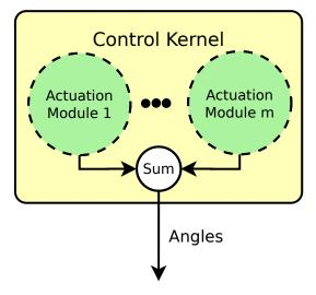
**Figure 4.4:** The control kernel contains all algorithmic modules calculating new desired positions for the joints of the robot. Several modules can easily be combined by summarizing their output. Using this technique simple locomotion can be extended with adaptive algorithms using sensor feedback.
