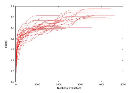
Figure 6.5: Maximum scores of 29 repetitions of GA-based amplitude optimization experiment.
