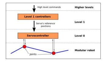
**Figure 5.1:** Concept of simulated servo controllers of the OpenRAVE-plugin OpenMR. As level 1 controllers several algorithms as actuation modules described on page 70 have been implemented. (González-Gómez [22])
