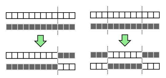
Figure 3.10: The principle of genome operation *crossover* is to swap sequences of genes between two genomes. Two genomes are necessary to perform this operation.
