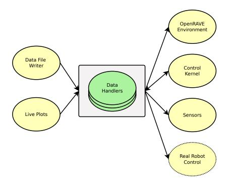
Figure 4.5: Data management is performed by several handler objects. Calculated data is appended to their buffers for live data observation and writing to files in a separate thread.
