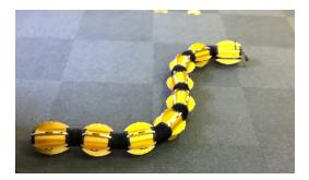
Figure 3.2: ACM-R5H is an amphibious snake robot. Efficient locomotion on land by using wheels is provided as well as swimming and diving in water. In both cases locomotion is generated by wavelike motions of the body. (HiBot [26])
