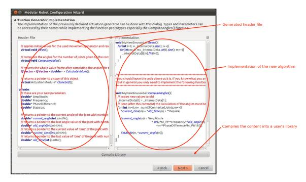
Figure 4.9: Actuation algorithm implementation is performed as second step. The main function that calculates the angular output has to be implemented as well as all helping functions. Then it gets compiled into the user library as a shared object file.
