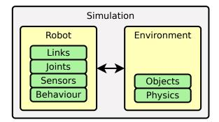
**Figure 4.2:** Overview of simulations. In simulations arbitrary configured robots interact with objects inside environments according to rules defined by the physics engine. Part of robots are the visible parts of their body as well as their behaviour and their sensing capabilities.
