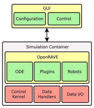
Figure 4.3: Main components of the system are the GUI and a simulation container. The GUI is divided into two different parts, one for configuration and one for control. In the container of the simulation the OpenRAVE-core is running as well as the control-kernel that controls the robot and all data handling.
