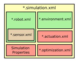
Figure 4.1: Structure of configuration files. Simulation configuration files include independent configured parts, like the robot or the environment. In this way components can easily be exchanged or reused.
