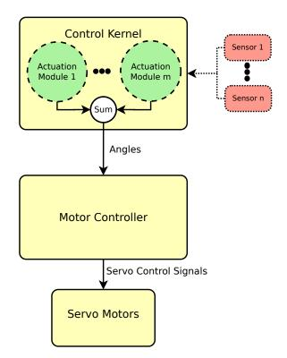
Figure 4.6: The control kernel with sensors in the big picture of the control system. Actuation modules have access to sensors if needed. In this way sensor information has influence on the angular output of the sum of control algorithms
