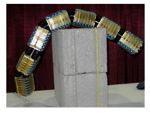
**Figure 3.4:** Each joint of Omni-Tread 4 (OT-4) is actuated by four independent pneumatic bellows. Locomotion is created by tracks. One of the design principles was to maximize the area of the robot covered by tracks. [44]
