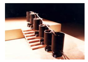
Figure 3.1: KORYU I is one of the first modular robots which redundant structure. By connecting several segments to a large chain it was able to climb stairs. In contrast single modules fail in this task. (Hirose [28, 29], Hirose and Morishima [30])
