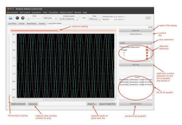
**Figure 4.21:** Data inspection tab helps to analyse data from files of passed simulation steps. After selecting a data file meta information is extracted about the content of this file and can further be selected for displaying or exporting. A nice feature is to capture directly screenshots of currently plotted data or to select desired plots for export to tab separated files.
