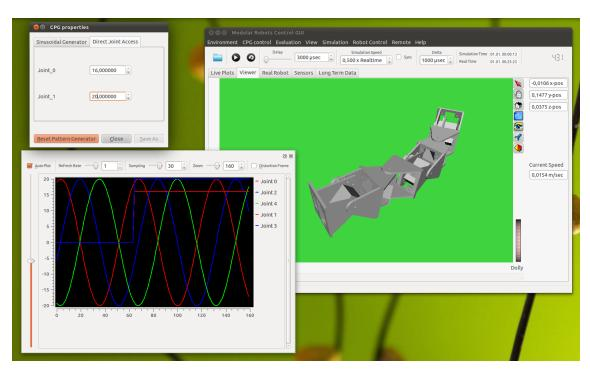
Figure 1.1: Example of the proposed system. The GUI of the control system is shown while operating a real robot. The simulated robot shows the desired state of the real robot. In the plot window the desired angles of the joints are displayed versus time. The small window in the upper left corner is used to change important control parameters.
