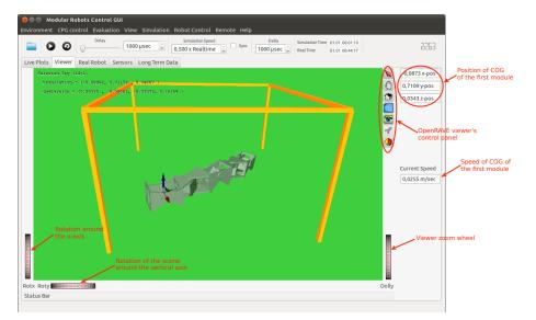
**Figure 4.19:** The environment viewer is based on the OpenRAVE viewer that has been integrated into the control GUI. OpenRAVE uses the Coin3d viewer for visualization of environments. To provide some additional useful information several GUI elements have been added that show the current position of the selected robot in the environment and its smoothed speed based on displacement.
