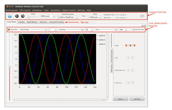
Figure 4.15: The main window of the control GUI enables users e.g. to supervise control algorithms with the help of live plots and the simulated environment by using the integrated coin3d viewer that is part of OpenRAVE.
