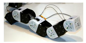
Figure 3.6: M-TRAN III is the third version of Modular Transformer. The limbless body generates locomotion with the help of waves travelling along the robot's body. These waves are generated by CPGs. The property of autonomous reconfigurability allows the robot to change its topology according to the needs to pass current obstacles. (Kamimura et al. [34])
