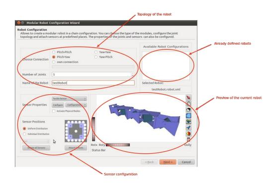
Figure 4.7: The wizard page for robot configuration is suggested to be used for easy creation of a robot. Joint topology can be adjusted and sensors can be placed at predefined places of the robot.
