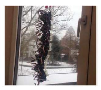
Figure 3.7: Climbing caterpillar-like robot (Chen et al. [11])
