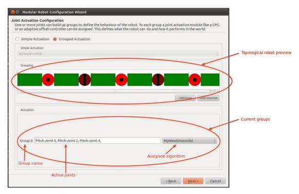
Figure 4.10: Assigning actuation modules to groups of joints creates the behaviour of a robot. Firstly, joints can be selected and grouped. Then one or more actuation algorithms can be assigned to a group.
