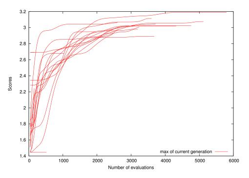
Figure 6.12: Maximum scores of 20 repetitions of irregular terrain experiment with GA.
