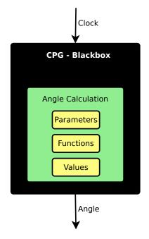
Figure 5.2: Each control algorithm that calculates angular positions of joints follows the concept of the actuation module blackbox. After receiving the command to calculate the next step angular output is generated. The function that produces the output uses previously in the implementation defined parameters, function and intermediate data.
