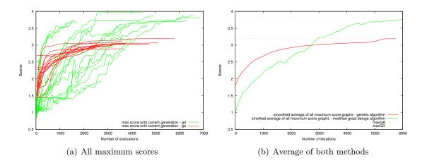
**Figure 7.2:** Comparison of learning rates in adaptive locomotion optimization. In (a) all maximum scores of each iteration of both experiments are shown. Red graphs represent scores of GA-runs and green graphs scores of GD-runs. Figure (b) shows the smoothed averages of both optimization methods. Red and green dotted lines mark largest distances reached by optimized parameters.
