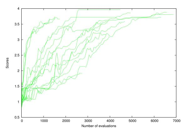
Figure 6.10: Maximum scores of 20 repetitions of irregular terrain experiment with modified GD algorithm.
