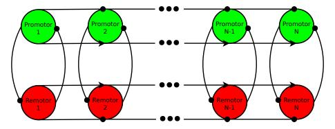
**Figure 3.9:** CPG network according to push-pull model introduced by Herrero-Carrón et al. [25]. Oscillators are composed of promoter and remotor neurons which are interconnected by inhibitory synapses bidirectionally. Unidirectional inhibitory and excitatory connections to next neighbours of promoters and remotors allow the whole net to synchronize. In this way a strong self-stabilizing network of oscillators is build that produces efficient locomotion patterns.
