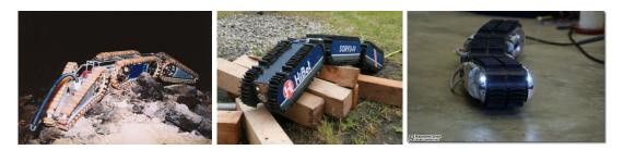
**Figure 3.3:** Series of Soryu robots consist of three modules driven by tracks. They are designed for tasks in rough terrain. Single modules can be autonomously disconnected or connected. These special joints are powerful enough to rotate or lift connected modules. (HiBot [26])
