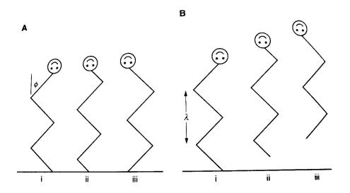
Figure 2.3: Illustration of the principle of serpentine movement. Maximum bending angle  $\phi$  and stride length  $\lambda$  determine frictional and inertial forces in serpentine movement. (Alexander [2])
