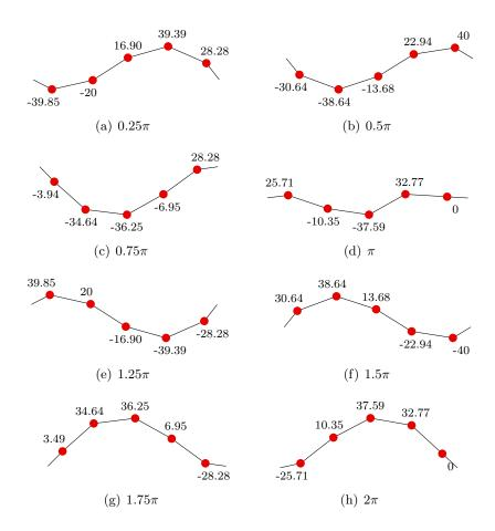
**Figure 6.1:** Different stages of a sine-pattern with uniform amplitudes applied to a chain of rigid links and joints. From (a) to (h) all stages of a whole locomotion cycle of  $2^*\pi$  is shown. The step-size between each stage shown is  $0.25^*\pi$ . The movements of the robot results in displacement from left to right.
