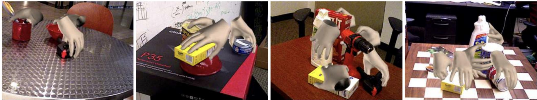
Figure 1: GanHand predicts hand shape and pose for grasping multiple objects given a single RGB image. The figure shows sample results on the YCB-Affordance dataset we propose, the largest dataset of human grasp affordances in real scenes.
