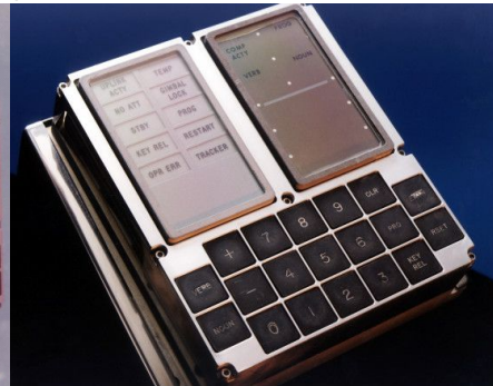
Dryden Flight Research Center EC96-45408-1 Photographed 1996 Apollo computer interface box used in the F-8 Digital Fly-By-Wire program. NASA photo by Dennis Taylor
