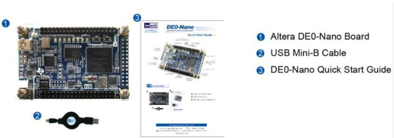
Figure 1-2 DE0-Nano kit package contents
