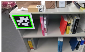
Figure: AprilTag detection is used to localize the shelf.
