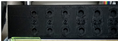
Figure: Working part tray with fixed size slots
