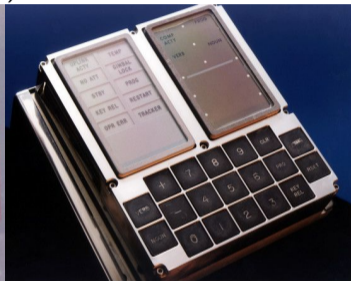
Dryden Flight Research Center EC96-43408-1. Photographed 1996 Apollo computer interface box used in the F-8 Digital Fly-By-Wire program. NASA photo by Dennis Taylor
