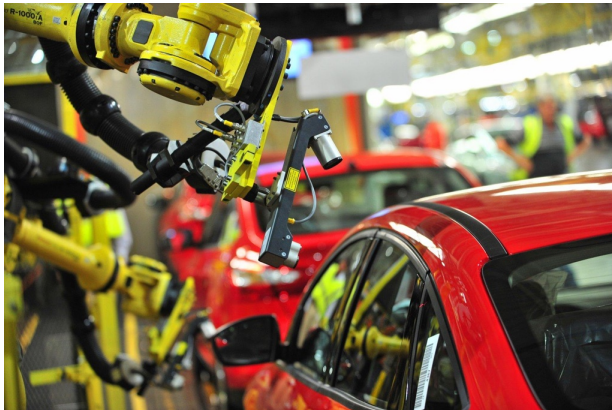
Automated visual inspection at the production line.
