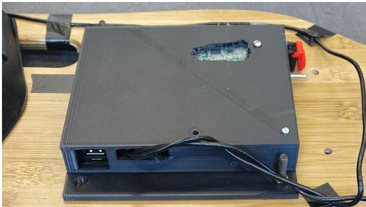
Figure: Eletronics box containing microcontroller, USB-battery, signal-amplifier and remote control
