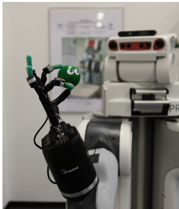
PR2 service robot with Shadow C6 electrical hand 19-DOF + 20-DOF gripper
