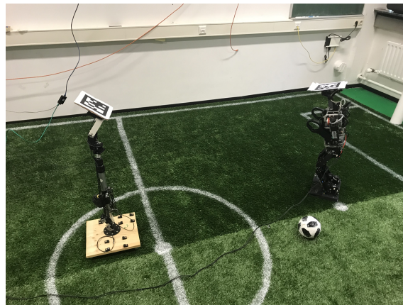
Figure 4.8: On the left, the camera used to record the robot. On the right, the robot. Not the AprilTag attached on top of both of them.
