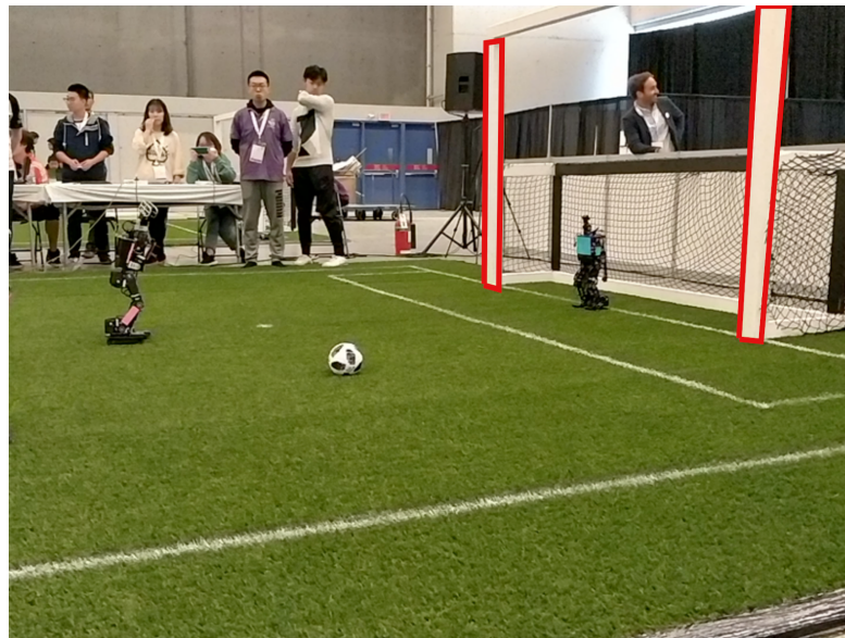
Figure 4.1.: Image from [2], edited to make label more visible. An example of manually labeled goalposts. The red outline encompasses the goalpost and will be used as ground truth for the training of the neural network.
