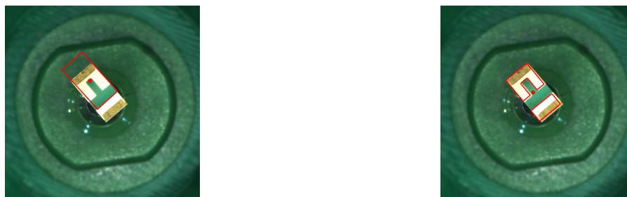
(a) Plain rectangular template matched to gripper image (b) Template with more details matched to same gripper image
