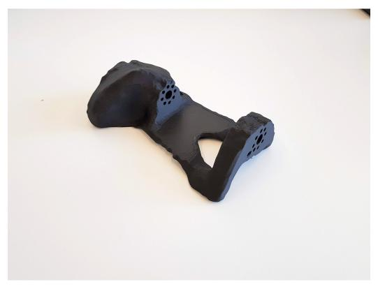
Figure 43: Printed optimized foot with screw holes of alternating depths making it impossible to mount
