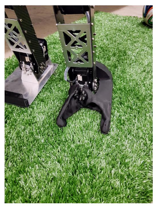
Figure 45: Optimized foot with only 15% mass retention setting mounted on the robot for a walking test
