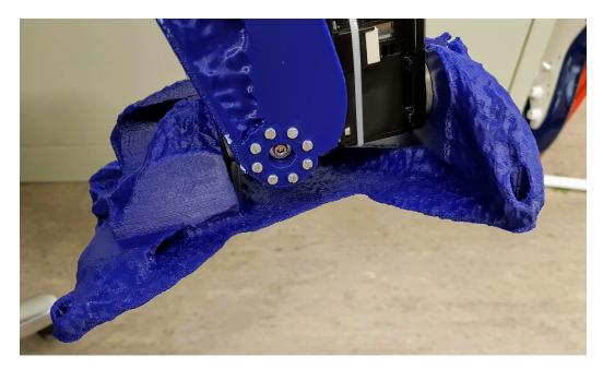
Figure 39: Side view of the printed optimized foot showing the connection to the leg
