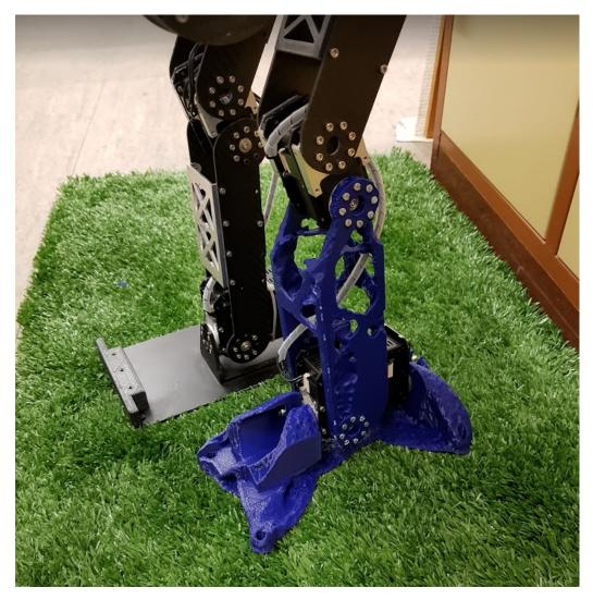
Figure 47: Optimized leg and foot mounted on the robot next to an unmodified leg
