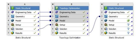
Figure 13: Workflow elements as seen in the ANSYS Workbench showing links between different steps of the optimization process
