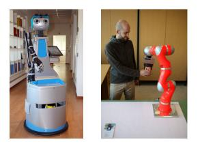
Fig. 1. The two robot systems used for the experiments: The *Domestic Robot* service robot designed for elderly care uses the Kinova Jaco arm (left). Our work cell setup with the KuKA LBR-4 in a robot-to-human handover task, shown with vertical gripper orientation (right). Our algorithm uses force and tactile sensor data to detect when to release the grasp.
