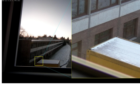
Fig. 6. In this image the PTZ-overlay function is shown. The ROI is chosen by the user. After the PTU, zoom and focus have been adjusted, the image is overlaid.
