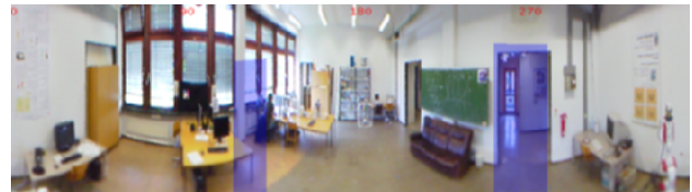
Fig. 7 Feature detector using laser range scan, the results are transformed to image coordinates for better visualization.
