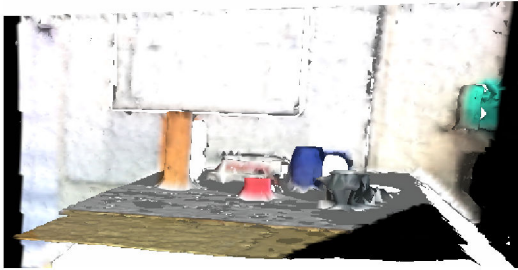
Fig. 13. The resulting reconstructed surface with the help of the Ball-pivoting algorithm from the colored point cloud. Only the fused area is presented.
