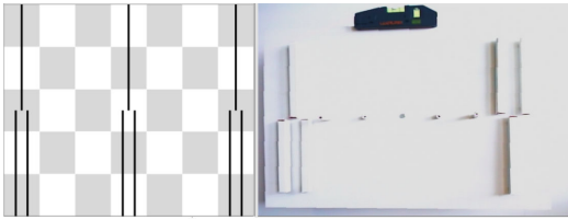
Fig. 8. The planned calibration pattern on the left and the 3D calibration pattern resulting from several experiments on the right.
