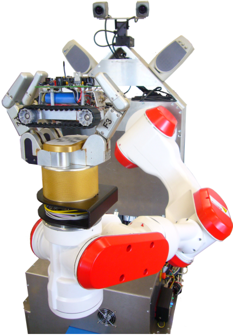
Fig. 3. Platforms used in the experiments: TASER's robotic arm is grasping small robot Lizard.
