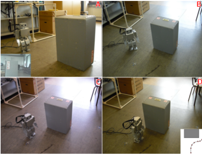
Fig. 11. Execution of the collision avoidance. The view of Hoap-2 by start and the resultant trajectory are displayed in the left lower corner of the image A and in the right lower corner of the image D.
