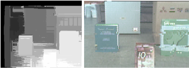
Fig. 6. Disparity map (left) based on the dynamic programming algorithm by Birchfield & Tomasi [14]. The brightness of an image point represents the depth of the real-world point. The brighter, the closer to the camera. A depth reconstruction (right) from the depth map is implemented by using OpenGL.
