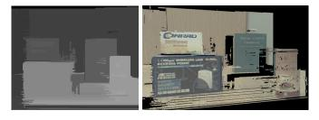
Fig. 9. Disparity map (left) based on the dynamic programming algorithm by Birchfield & Tomasi [22]. Brightness of an image point represents depth of real-world point. The brighter, the closer to the camera. A depth reconstruction (right) from the depth map is implemented by using OpenGL.
