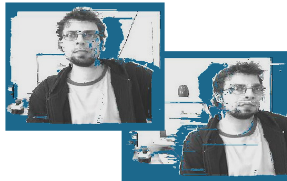
Figure 10: Two virtual views of a reconstructed face based on the disparity map of Fig. 9.
