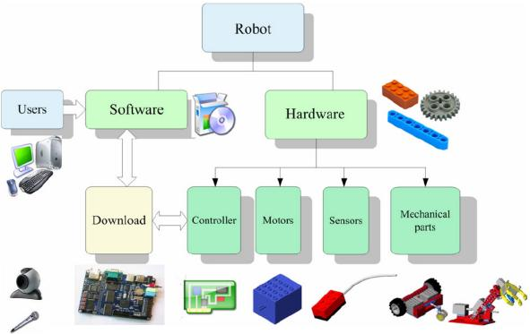
Fig. 1 Block diagram of our new tutoring system for the practical course
