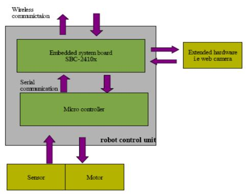
Figure 12: The communications structure.
