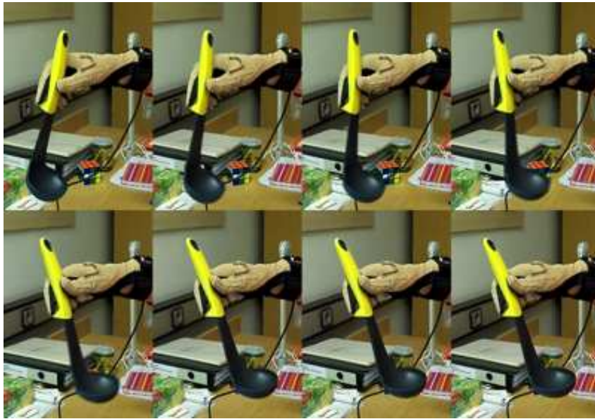
Figure 42: In-hand rotation of a ladle. Thumb, first and middle finger participate in this scenario, the ladle is moved to a higher position and this process is defined as a trial
