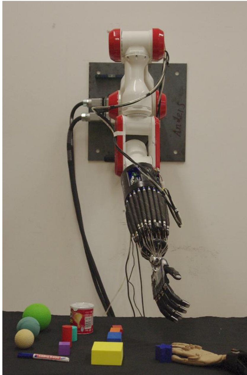
Figure 1: The experiment setup in Hamburg, with the Shadow air-muscle hand mounted on the PA-106C robot arm and tele-operated via the CyberGlove-II. The objects on the table are from the IST object set (compare section 3.1). A Kinect sensor is mounted below the robot base; the multi-camera system is not shown.
