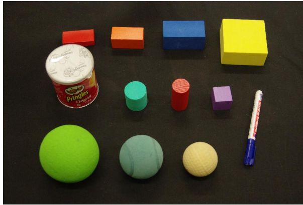
Figure 13: The set of prototype objects suggested by IST. The objects include three basic shapes (sphere, cylinder, box), different object diameters matched to typical human grasping tasks, and different materials (sponge, rubber, wood, metal).
