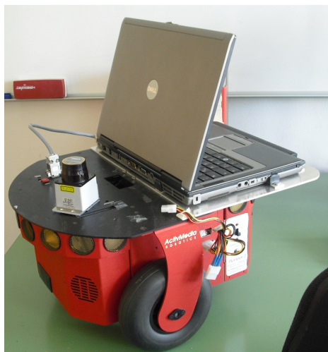
Fig. 3.2: A Pioneer robot used in this work. The mounted laptop runs the control program and communicates wirelessly. The (dismounted) laser can be seen on top of the robot and the fixed sonar sensors are visible as circular devices underneath the top board at the front.
