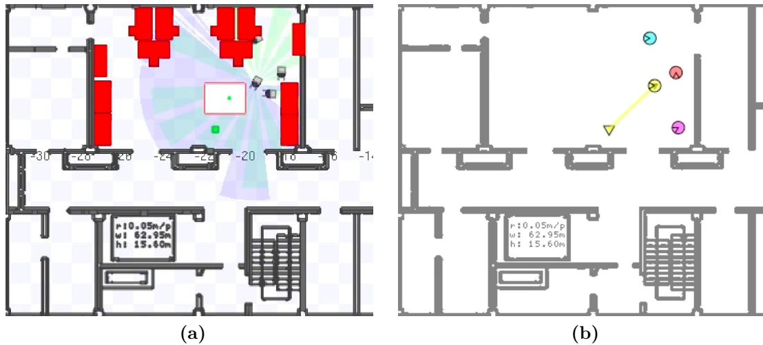
Fig. 4.6: Another event within the same run of the Find and Collect scenario depicted in figure 4.5. (a) Virtual environment view. The event of the searching robot detecting a green blob within its field of view (white square in center) is depicted. Communication regarding the newly found target is triggered. (b) The collector robot listens for such targets and has planned a path to the target, shown here in the planner view.
