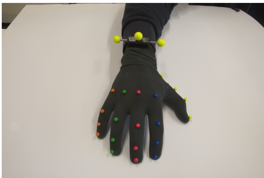
Figure 5.3: The glove design using colored, passive marker objects to approximate the joint positions. Different colors were used to simplify the identification of the joints in the kinematic chain of each finger.
