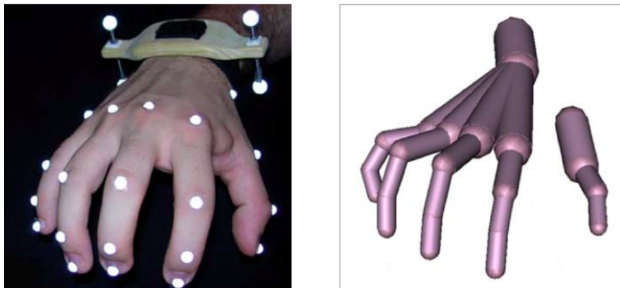
Figure 1.3: The hand equipped with retroreflective marker objects (left) used in the approach by Cerveri et al. [CDML + 07] and the reconstructed three-dimensional model (right).
