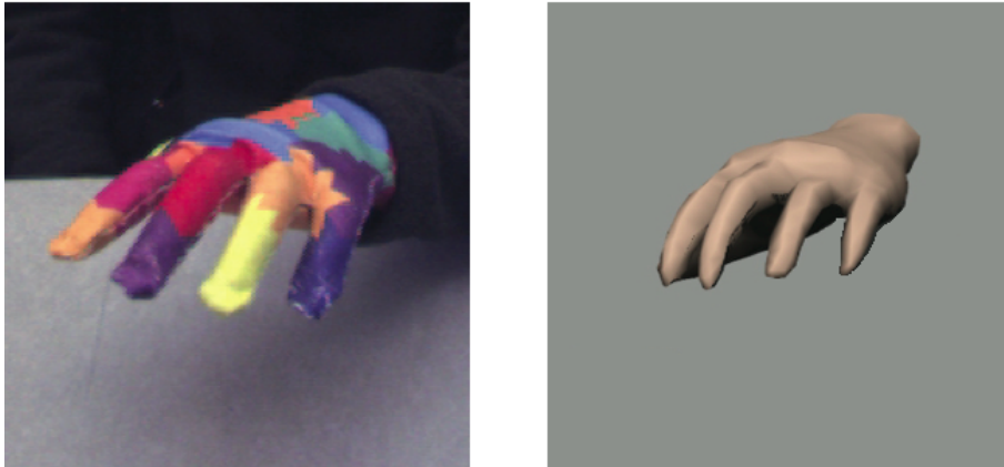
Figure 1.2: Colored glove (left) used in the approach by Wang and Popović [WP09] and the reconstructed three-dimensional model (right).
