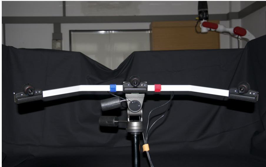
Figure 5.2: The three-camera stereo vision setup. Three PlayStation® Eye cameras were mounted in a convergent configuration. The red marking signified the first stereo pair, while the blue marking signified the second stereo pair. The length of the baselines was determined as 331.0562mm and 331.7844mm, for the first and second pairs respectively.
