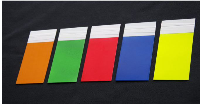
Figure 5.4: The color sample plates. The plates were used for the purpose of calibration of initial estimates for the thresholds of each color.
