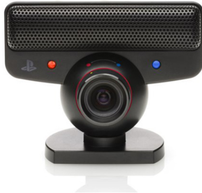
Figure 5.1: The PlayStation® Eye camera used in the experimental setup. The camera offers a maximum frame rate of 60Hz at a resolution of 640 \times 480 pixels. The factory fixed-focus zoom lens offers two levels of magnification with a field of view of either 56^\circ or 75^\circ . The upper segment of the camera contains an array of four microphones.
