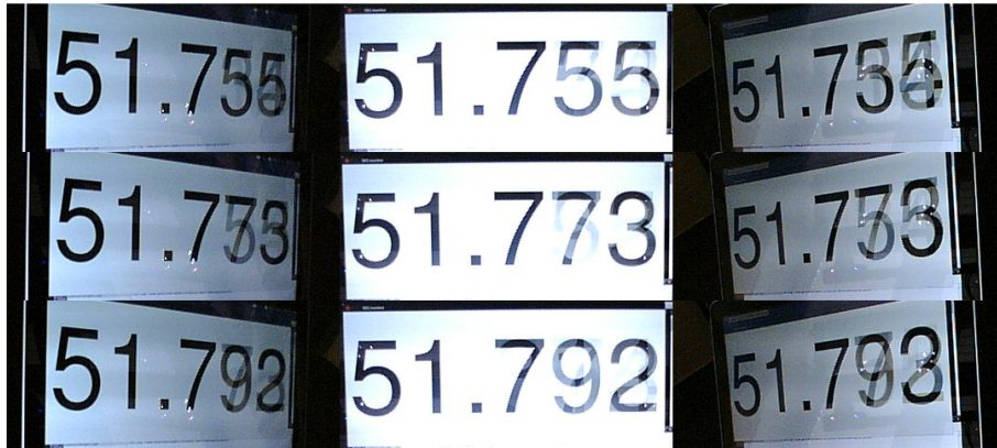
Figure 6.1: Three image sets from the recorded sequences of a counting timer (milliseconds). The image sets are displayed from top to bottom, with the images of each single camera from left to right.
