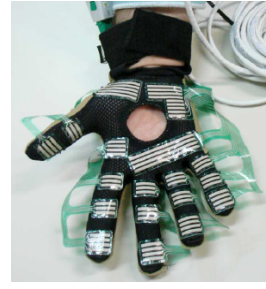
Fig. 7. The experimental setup for hand pose and tactile information acquisition [24]. The demonstrator wears the Cyberglove for the hand posture sensing. The front side of the hand equipped with a Tekscan Grip system receives the contact information.
