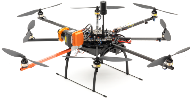
Fig. 1. The experimental flying platform with mounted GNSS-antenna/receiver, processor-board, laser scanner and IMU.
