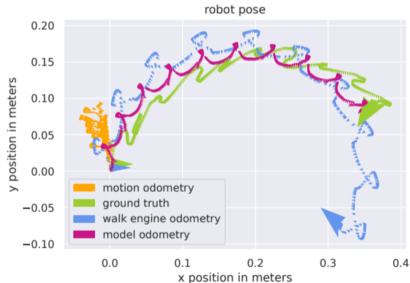
Quiver plot of the odometry approaches using SimNet on simulation data.
