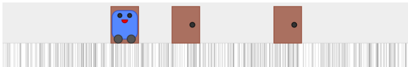
Fig. 4: Upper part shows the illustrated environment. Lower part the uniformly distributed amount of particles
